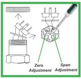
For potentiometer clockwise direction to increase anti-clockwise direction to decrease
