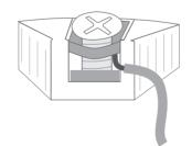
Wires must be mounted between the metal plates.
