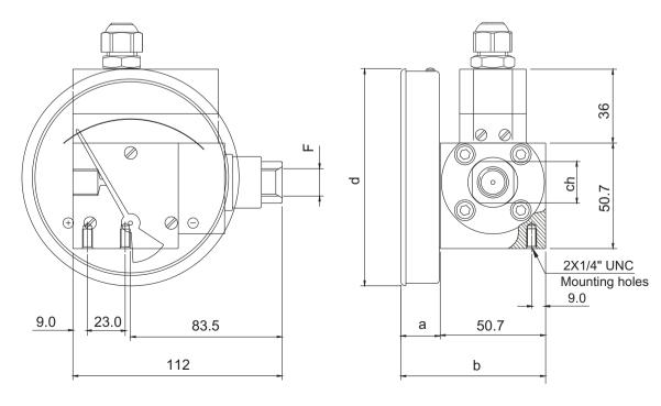
Gauge + Switch with reed contacts with teminal strip & 1/2" conduit connection
